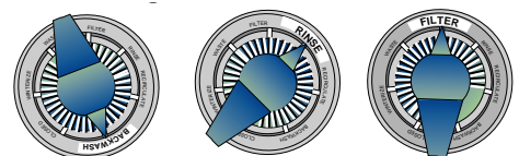
Fig. 9: Valve settings for startup. Stop pump before changing valve position.
